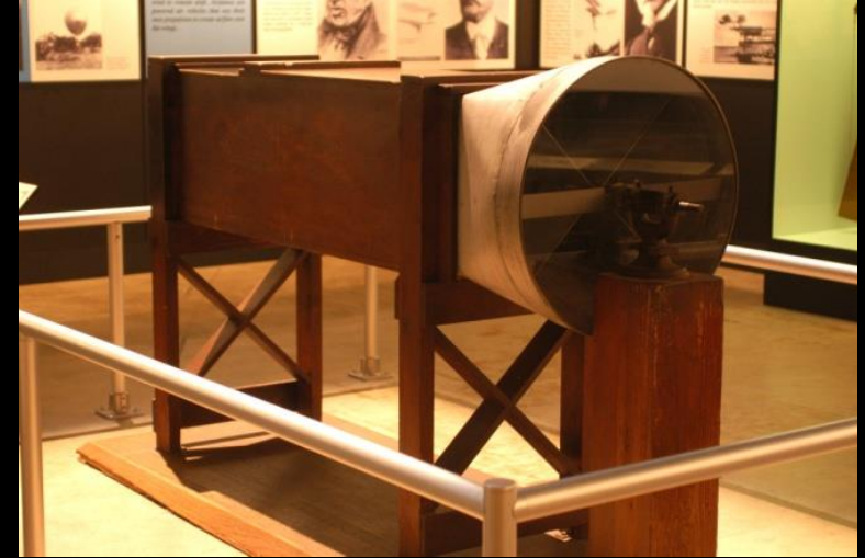
1901 Wright Brothers' wind tunnel. By matching dimensionless parameters in scale-models we get reliable predictions of behavior.
