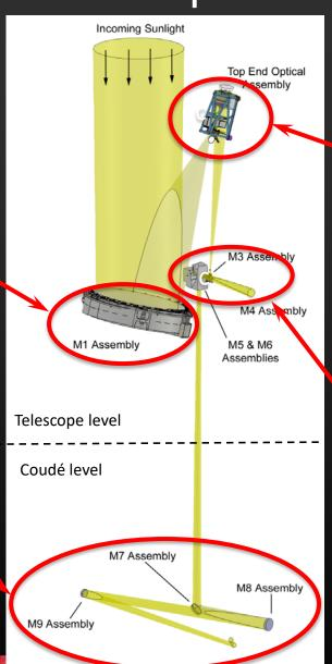
Top End Optical Assembly (TEOA) - The TEOA contains the 62 cm M2 mirror, the Heat Stop Assembly (HSA), the Lyot Stop, the M2 Support Frame and associated control systems.
