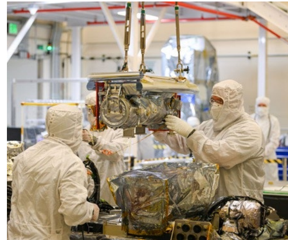
CCOR-1 integration onto GOES-U
