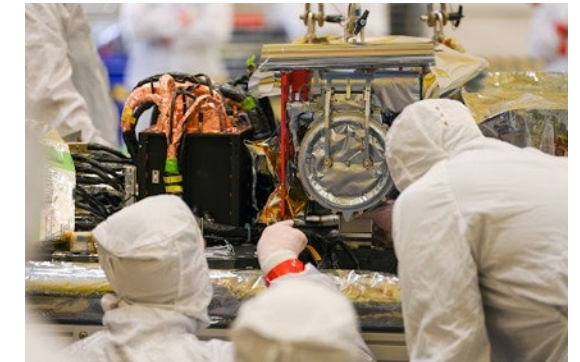
CCOR-1 integration onto GOES-U
