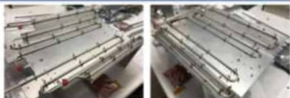
RTG Heat Exchanger Hot Plate Tube Bending
