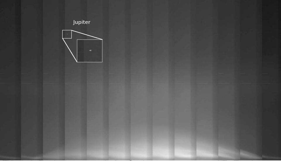
This single-filter image was acquired on October 9, 2013 at 18:51:30 UT. The glow at the bottom is scattered light coming from the earth, just outside the camera field of view.
