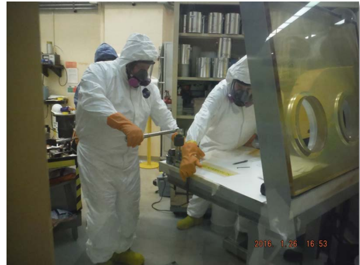
ORNL Staff close the middle package using a torque wrench
