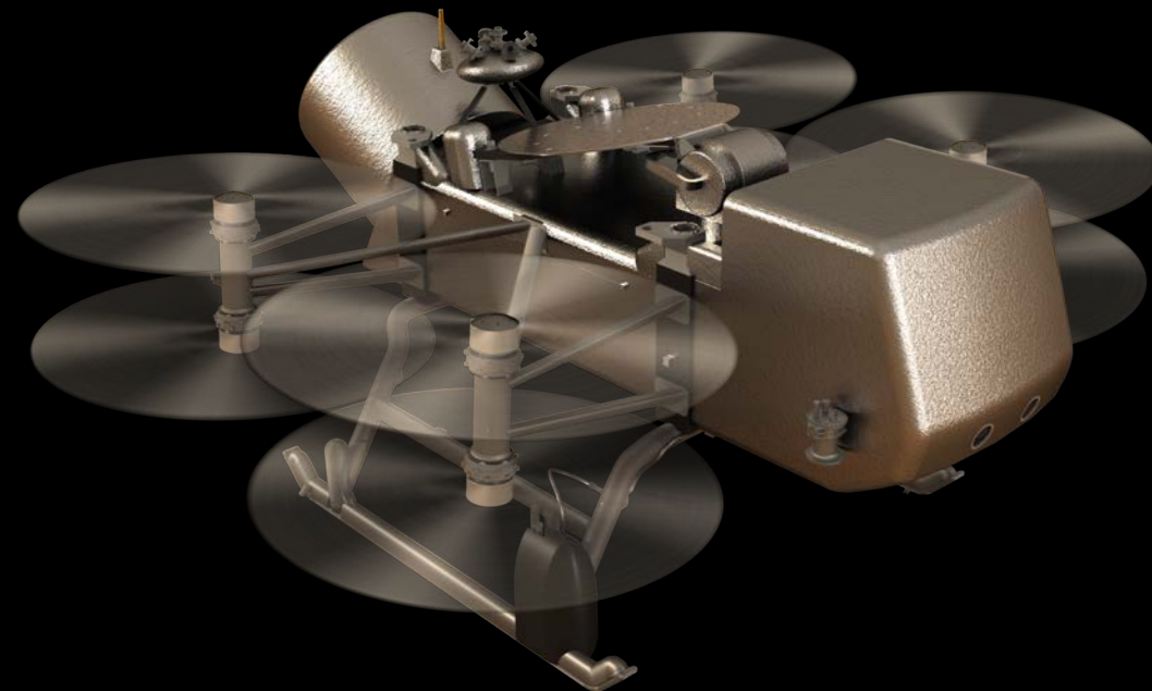
Rotorcraft Lander Flight configuration with HGA stowed
