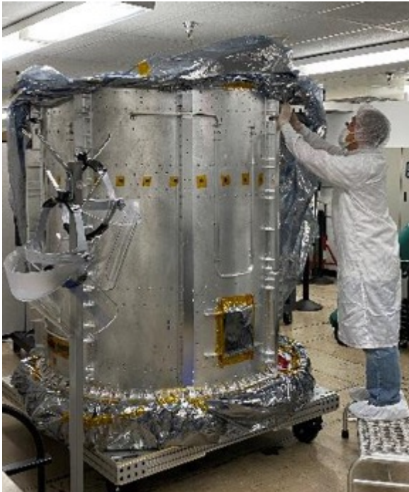
Above: Upper cylinder of propulsion module
