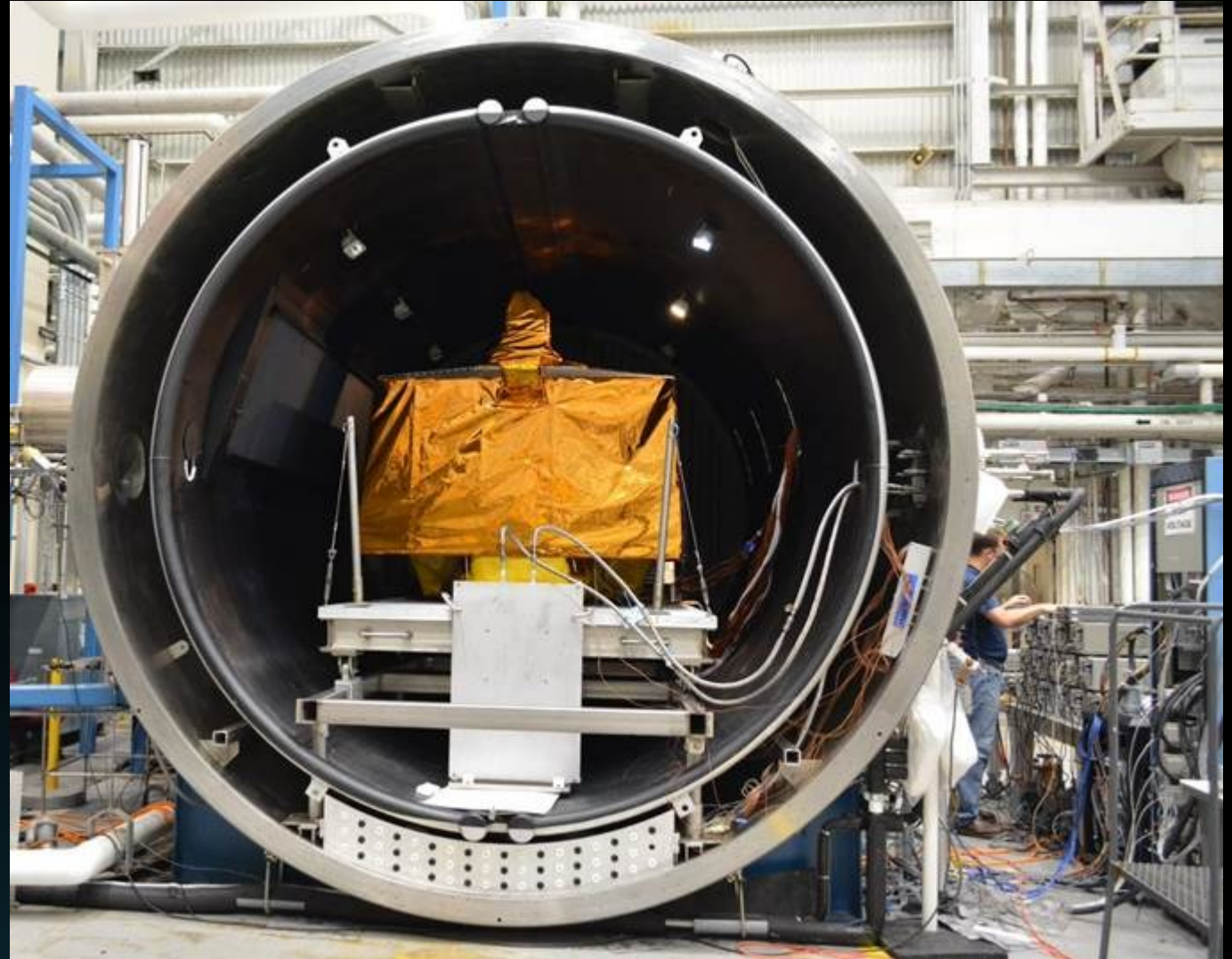
Rover thermal test unit in TVAC at MSFC
