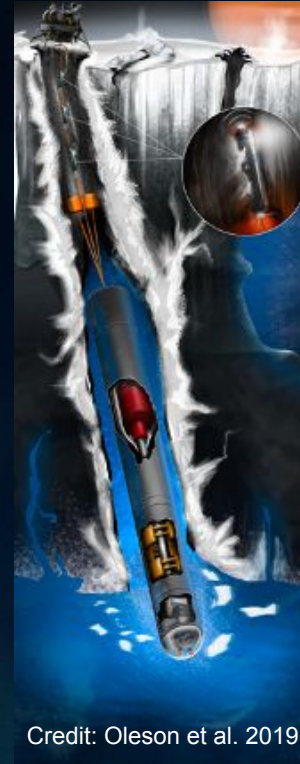
Fig 2. Artist concept for a cryobot probe
