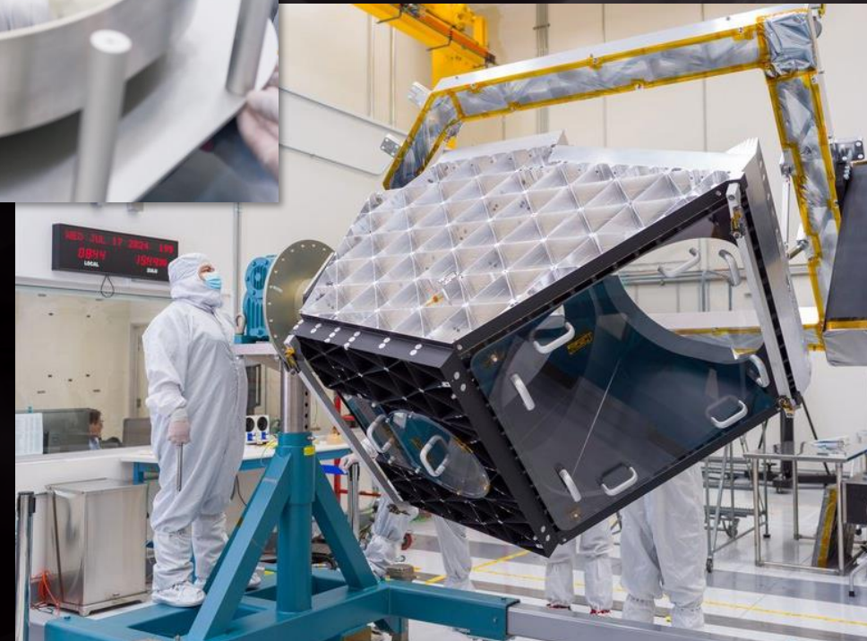
NEO Surveyor mirrors undergoing inspection (top) and telescope optical bench under construction (right) at JPL, August 2024
