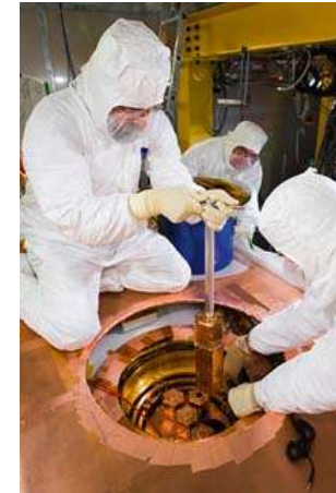
Cryogenic Dark Matter Search (CDMS) at Soudan mine - germanium detectors - operating
