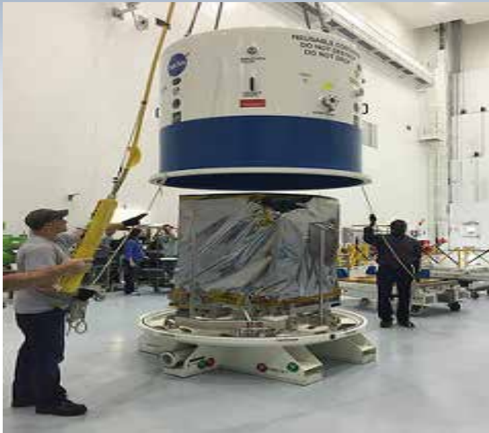
Removal of shipping container cover from NICER payload at Kennedy Space Center
