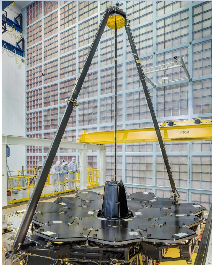
Completed Optical Telescope Element (OTE), with secondary mirror and Aft Optics Assembly (AOS) installed, at GSFC SSIDF.
