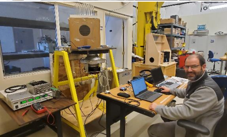
Assembly & testing of M1M3 fan-coil units
