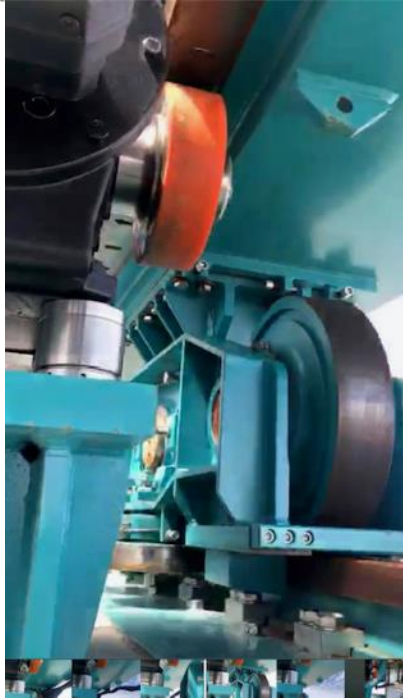
Friction-drive rotation system Implemented
