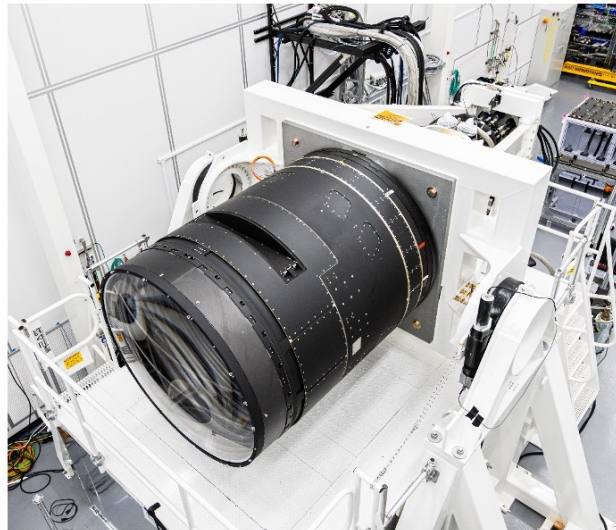
Camera showing L1 lens
