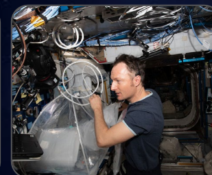
ESA astronaut Matthias Maurer works on the Concrete Hardening experiment
