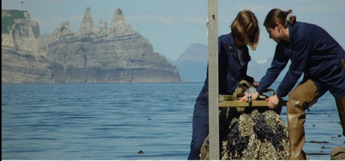
Two women wearing rubber boots, standing on rocks at the shore and installing a tide gage instrument.
