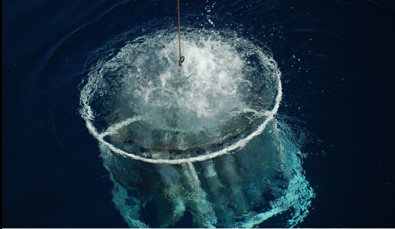
Conductivity, Temperature and Depth (CTD) sensor being lowered into the ocean with air bubbles at the ocean surface
