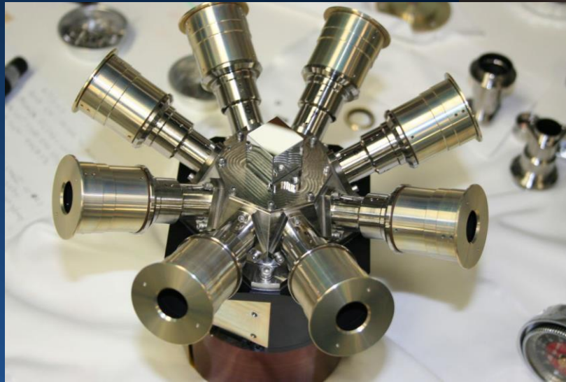
ARGOS flight hardware. Note the eight apertures arrayed around a central optical hub containing the prism. (credit: M. DeLand)
