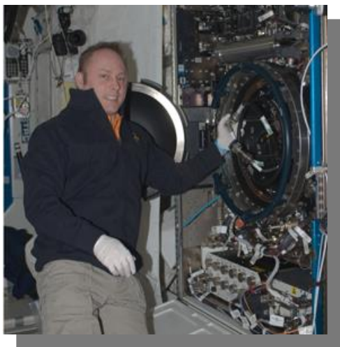
COMBUSTION: Astronaut Mike Fincke completing install of the CIR/MDCA insert prior to CIR activation in January 2009.
