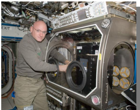
COMBUSTION, FLUIDS, COMPLEX FLUIDS, MATERIALS, BIOPHYSICS: Increment 26 commander Scott Kelly installing CCF in the Microgravity Science Glovebox ( MSG ) on ISS
