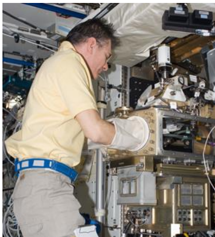
FLUIDS, COMPLEX FLUIDS, BIOPHYSICS: Astronaut Paolo Nespoli operating the ACE experiment in the FIR/LMM
