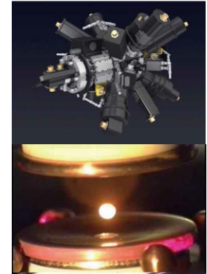
Top: model of ELF hardware Bottom: levitated sample in the ELF ground unit
