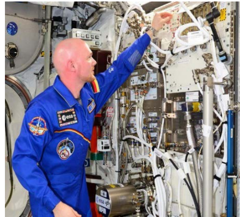
Electromagnetic Levitator Furnace MATERIALS: Investigate thermophysical properties of metal alloys. Astronaut Alexander Gerst completing installation of the ESA (with DLR) EML , October 2014 on ISS
