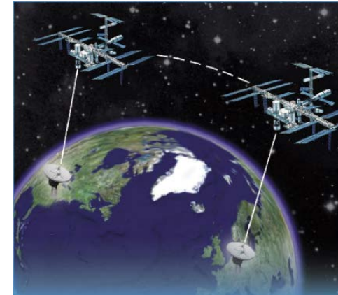
Atomic Clock Ensemble in Space. Time measurements made at various locations around the world with atomic clock on the ISS. ESA to provide two microwave link ground stations for NIST and JPL.
