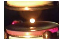
Levitated sample in JAXA's ELF ground unit
