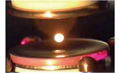
Levitated sample JAXA's ELF ground unit
