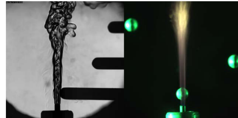
Co-flow fuel jet, 30% \text{C}_2\text{H}_6\text{O} (aq) in core and air in annular region injected into bulk SCW reactor
