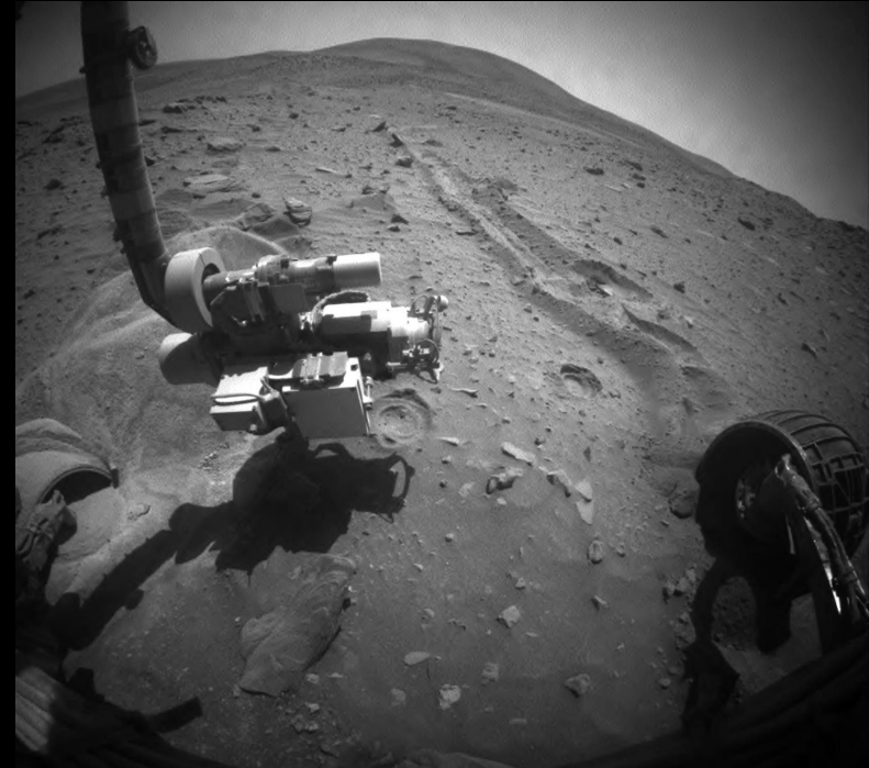
Self-portrait of the rover Spirit stuck in a Martian sand trap (2009) NASA/JPL-CALTECH
