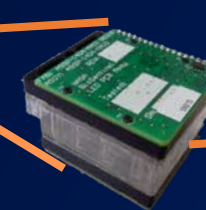
Biosensor payload with fluidic cards and optical sensors
