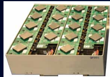
Biosensor payload with fluidic cards and optical sensors
