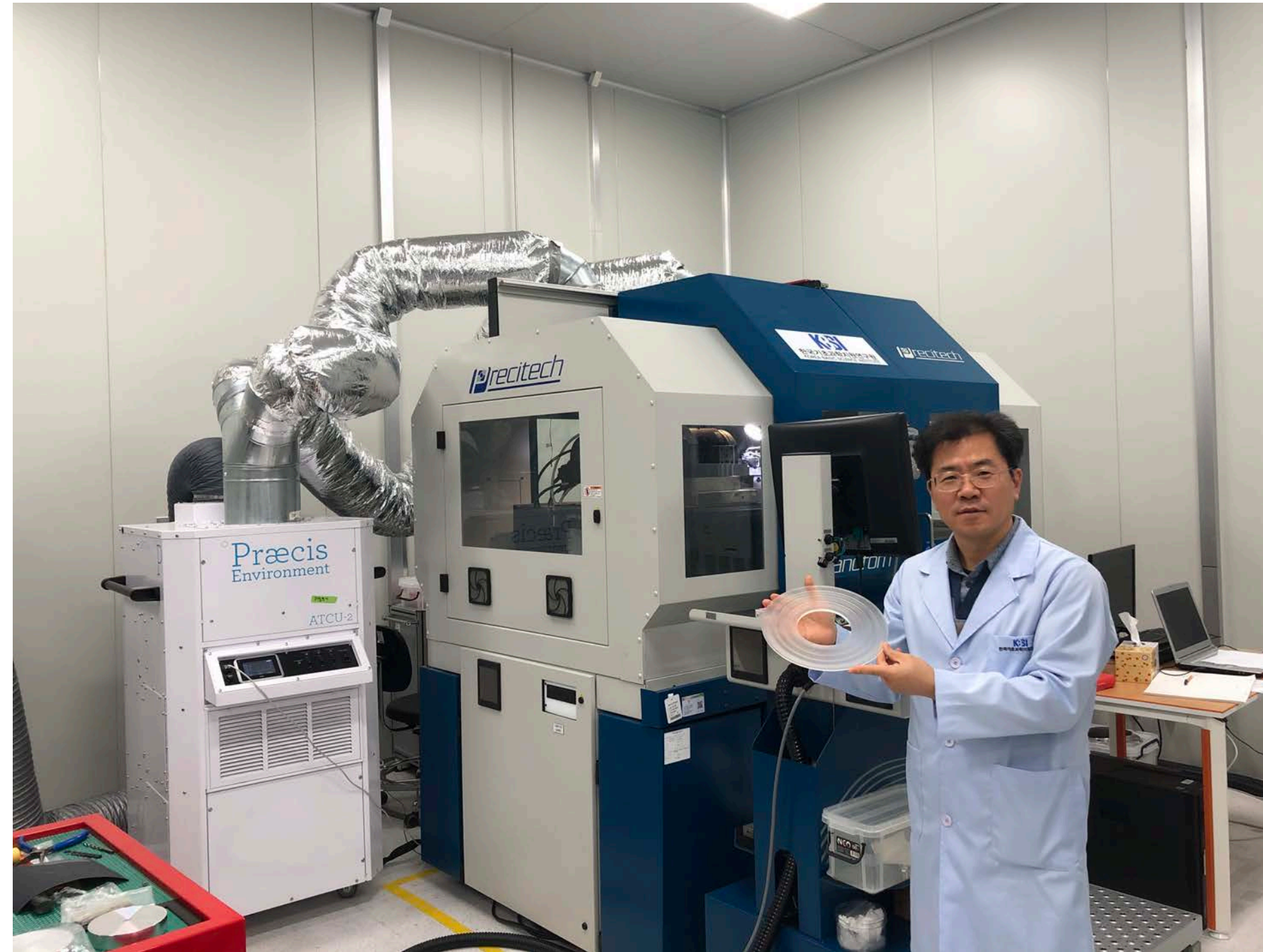
High-performance diamond turning machine with ultrasonic tool vibration upgrade at KBSI
