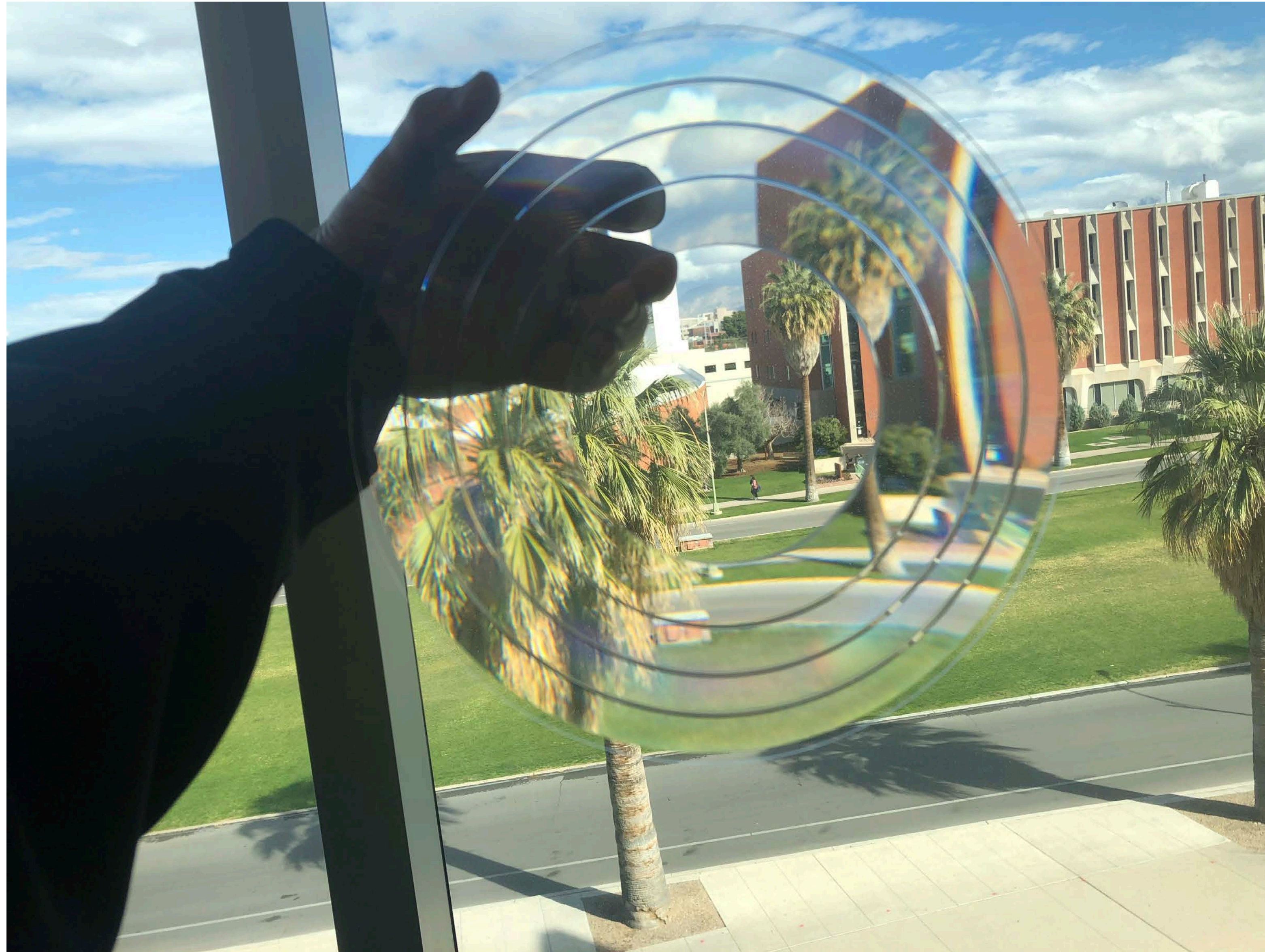
PMMA prototype diamond turned at KBSI
