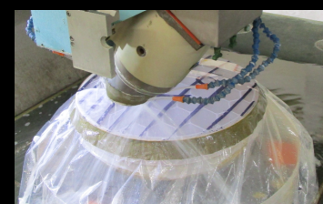
In process shaping of SM to WFIRST prescription
