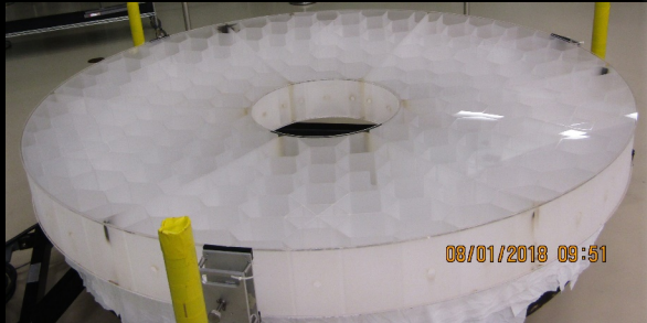
Flight Primary Mirror As received
