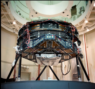
Primary Mirror Assembly + Forward Metering Structure At SRR/Pedigree Review
