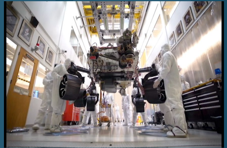
Oct. 8, 2019 – Engineers, at NASA's Jet Propulsion Laboratory, lower the Mars 2020 rover to carry its full weight for the first time
