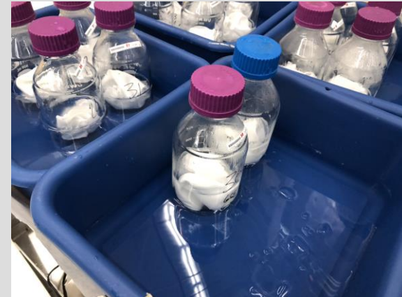
Quenching shocked samples in ice bath
