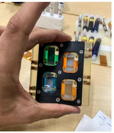
A preflight photo of the BioCell bioreactor for housing engineered muscle developed in collaboration with BioServe Space Technologies.
