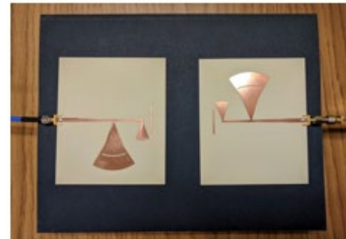
RF Power Harvesting Antennas- UAH
