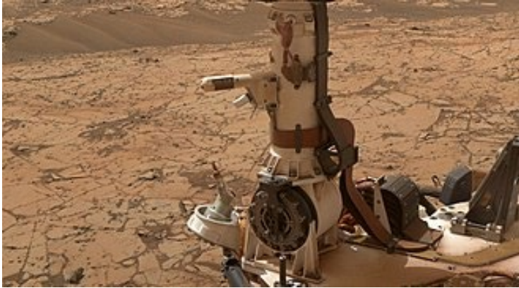
Rover Environmental Monitoring Station (REMS) on Curiosity (NASA/JPL/Caltech)
