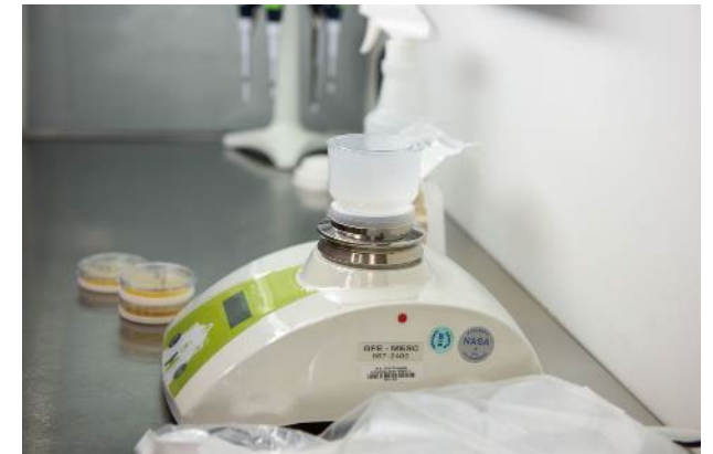
Membrane filtration setup.
