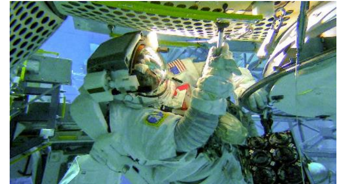
NASA Image: JSC2023E026248 - NASA astronaut Victor Glover tests hardware for the ISS External Microorganisms investigation at the Neutral Buoyancy Laboratory at NASA's Johnson Space Center in Houston.
