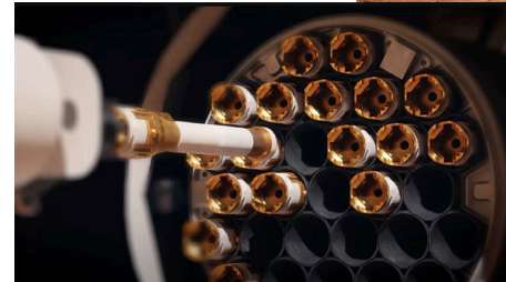
At Left - Close up of sample tube installation into the OS by the Sample Transfer Arm. During installation, the OS exterior and interior are exposed to wind blown Mars dust. When tube loading is finished, the particle-tight OS lid is installed, containing the samples and much of the dust inside the vessel. Exterior dust is later subjected to sterilization in space.
