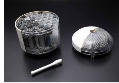
At left - A sample tube and the Orbiting Sample container (OS) and lid in which tubes would be launched from Mars. Above - the Mars Launch System with the closed OS on the front (arrow)
