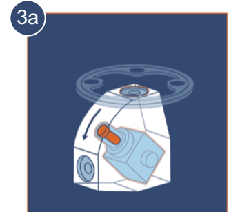
3a Bit Carousel pivots , the Airlock door is closed and, then motion is paused to settle any dust.
