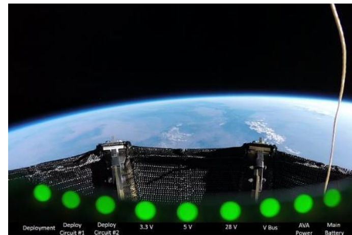
ARC successfully flew a 70 cm diameter ADEPT skirt on a suborbital sounding rocket
