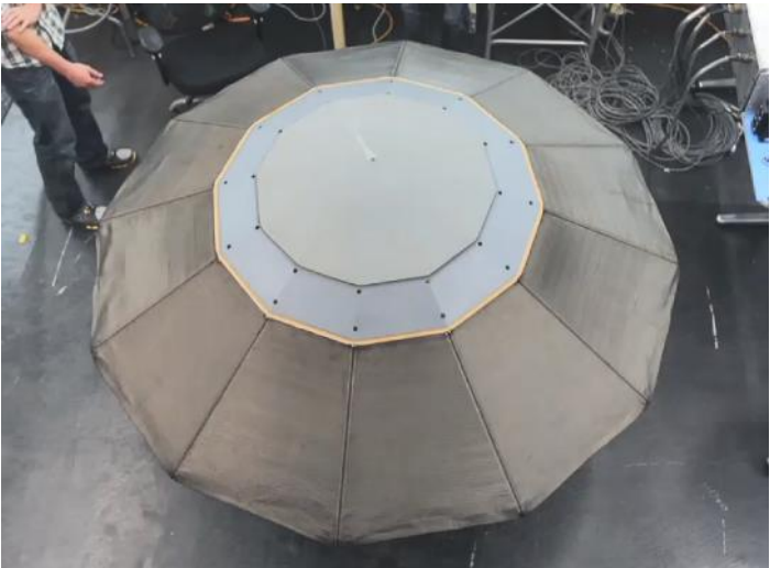
Electrically driven actuators achieve high fabric pre-tension
