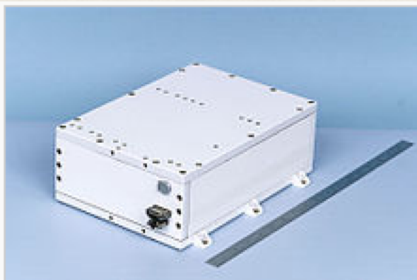
MARIE, designed to measure radiation, started malfunctioning shortly after a series of strong solar flares occurred in Autumn of 2003
