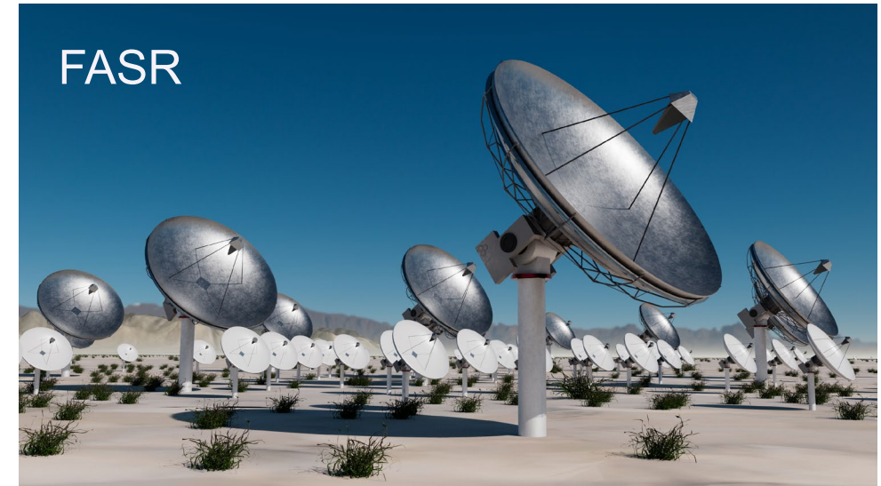
FASR MSRI-2 ($20-100M): Frequency Agile Solar Radiotelescope – A 3D radio “camera,” observes the Sun’s atmosphere as a coupled system
