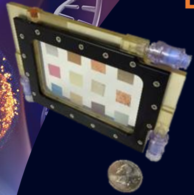
BioCell used in biofilm experiments on the ISS
