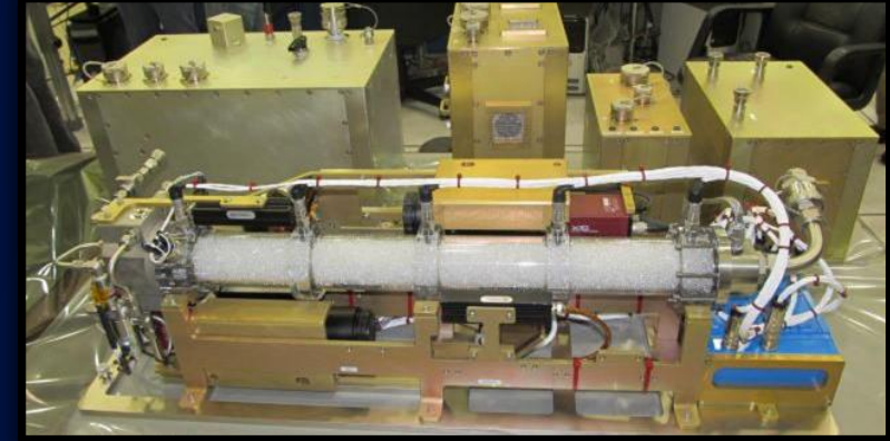
PBRE-2 test column with 2mm glass beads
