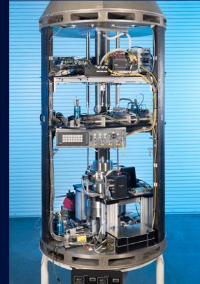
High Pressure Transcritical Combustion Facility: shown in drop "vehicle" in drop configuration (L) and close-up of Droplet Module Insert used for high pressure droplet combustion experiments.
