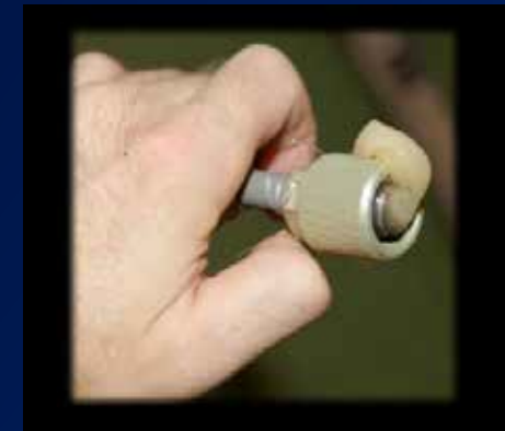
Extensive biofilm formation in ISS water recovery system
