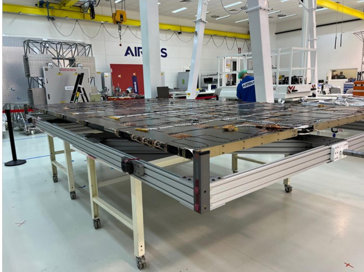
Integration of Solar Panel PX P1 completed (with exception of the REASON antenna)
