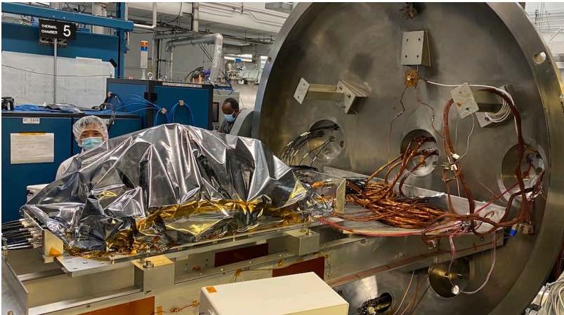
REASON Electronics in TVAC
