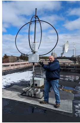
New high-rate real-time GNSS receivers installed for the eclipse experiment in numerous locations from Texas to Vermont – in farm fields, backyards, and football fields
