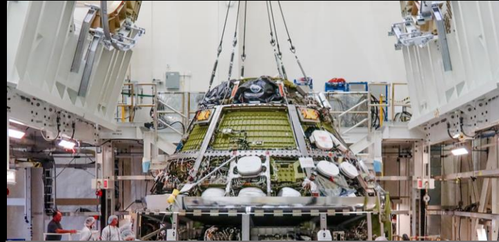
Integration of Crew and Service Modules for the Artemis II Orion Spacecraft
