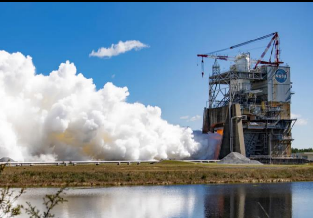
Certification testing for production of new RS-25 Retrofit 3b engines to power the SLS rocket, beginning with Artemis V, completed early April 2024
