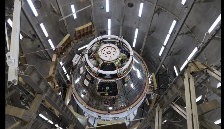
Artemis II Orion Spacecraft inside the altitude chamber at NASA's Kennedy Space Center for testing
