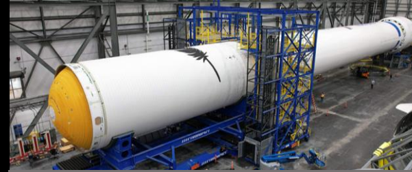
The first and second stages of New Glenn's test vehicle mated for the first time enabled Blue Origin to exercise their tooling and stage interfaces in preparation for the first launch.
