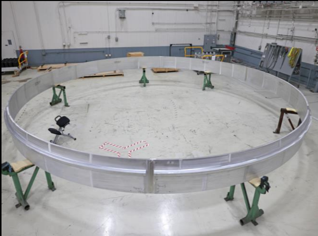
Artemis V Y-ring manufactured at Michoud Assembly Facility
