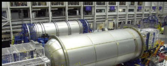
Hardware for Blue Origin's New Glenn second stage, which will refuel the cislunar transporter as part of Blue Origin's Artemis V architecture, is being manufactured at Blue Origin's production facility in Cape Canaveral, FL.
