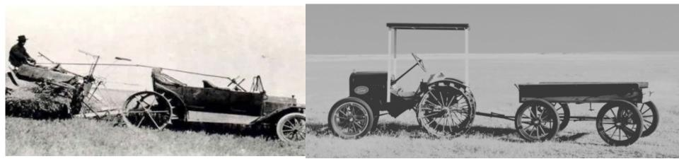
Torque + Grip + Weight = Traction & Reaction for Work Mobility increases and sinkage decreases with increased radius & Rim width Soft suspension of a rover for driving around is counterproductive to a work mahine for loading, grading, lifting & assembly
