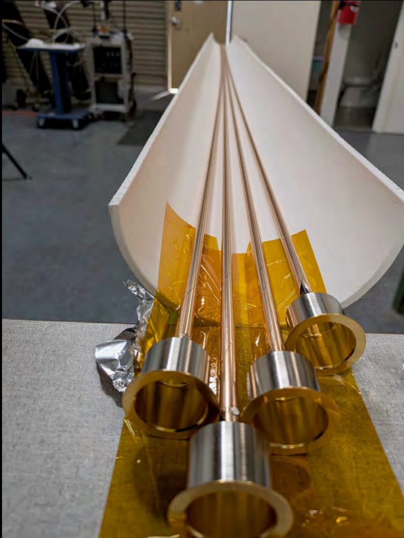
Rolled BeCu sheet, Stowed during launch, deploy as rolled flat spring
