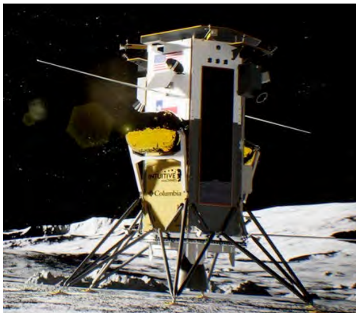
IM-1 with ROLSES antennas deployed
