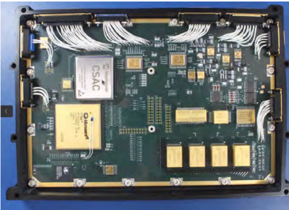
Digital Control Board for LuSEE-Night
