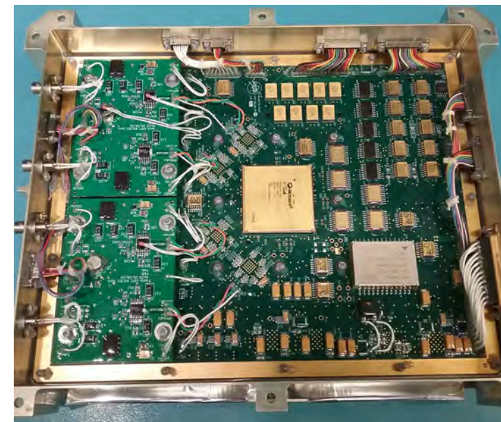
ROLSES spectrometer board
