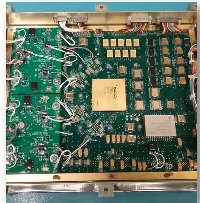
Spectrometer board with FPGA
