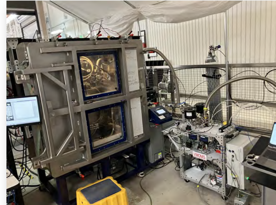
MRE undergoing testing in a vacuum chamber at NASA KSC
