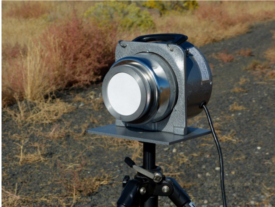
High volume sampler (15 ft 3 /min)
