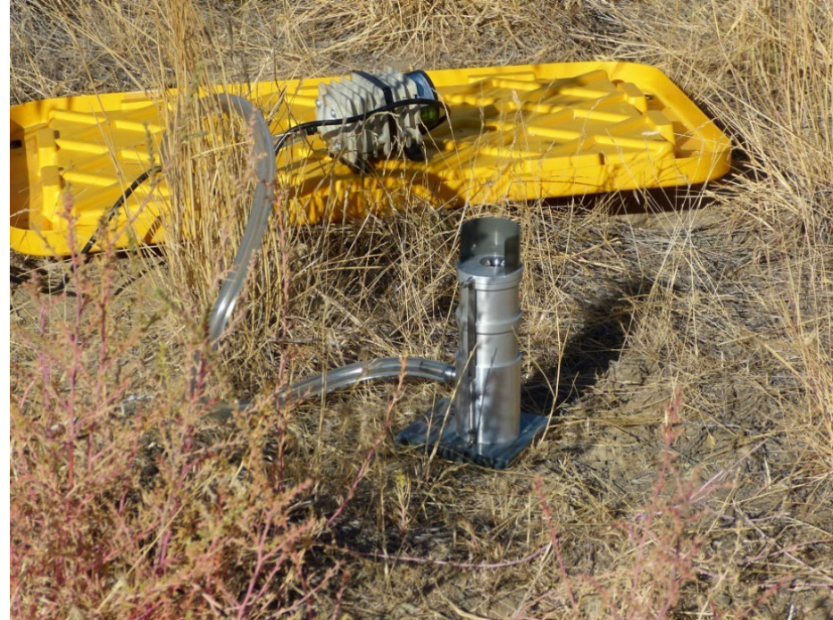
Burkard multi-stage liquid impinger (0.46 ft 3 /min)
