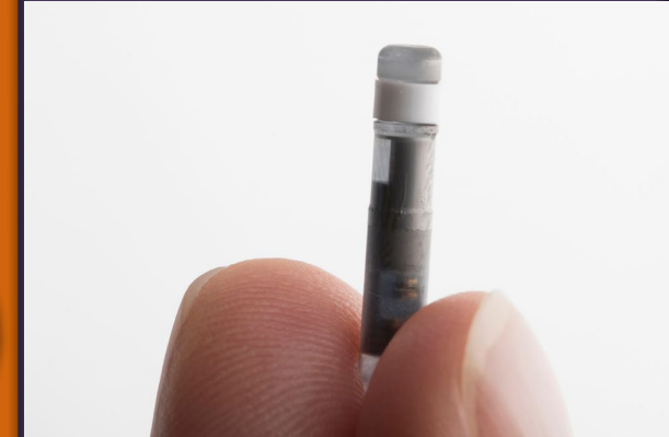
Eversense implantable CGM (Senseonics)
