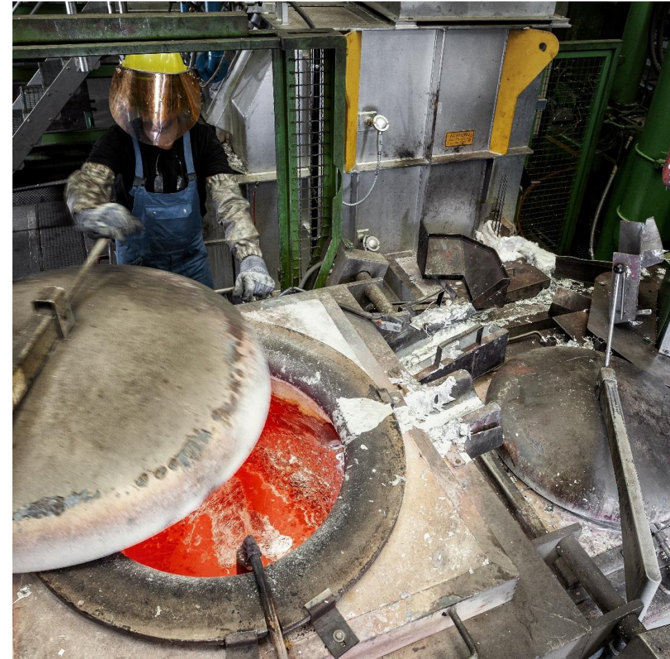
Worker preparing materials for die casting
