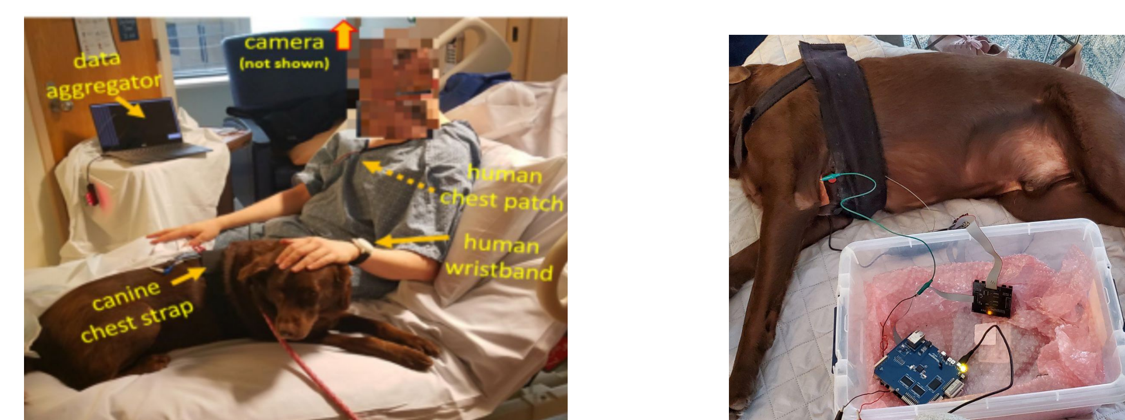
Figure 3. (Left) The measurement set up with subjects wearing wireless sensors (Right) Non contact electrodes placed on dog to track sleeping behaviors. .
