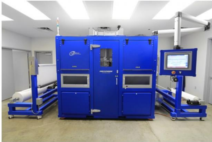
FibeRio's Forcespinning technology is capable of both melt and solution spinning nanofibres. © FibeRio Technology Corporation
