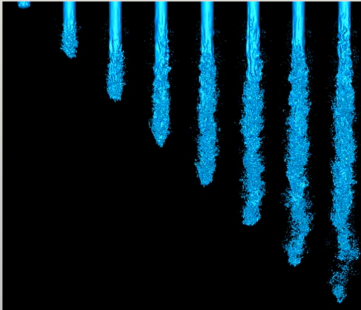
Turbulent spray breakup
