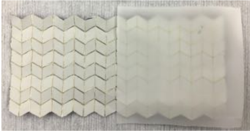
1. Insert nanoporous membrane sheet between two laser-patterned foils
